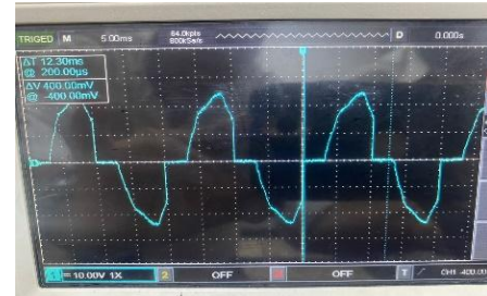
Fig 20. The THD for the Voltage
