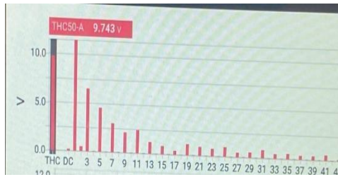
Fig 18. The THD for the Voltage
