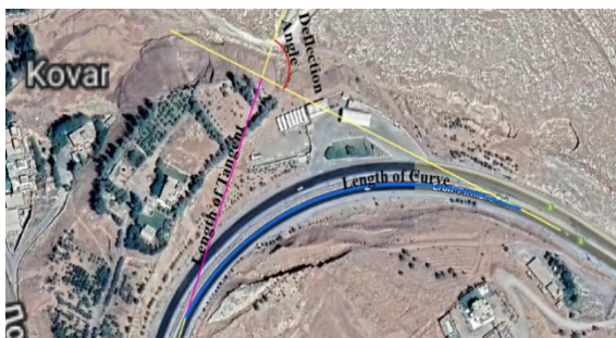
Fig. 2 Horizontal Curve Elements.
